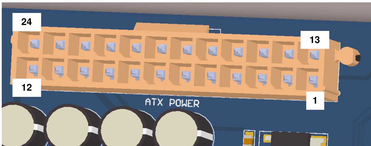
Figure 4 – P1 ATX Power Connector
