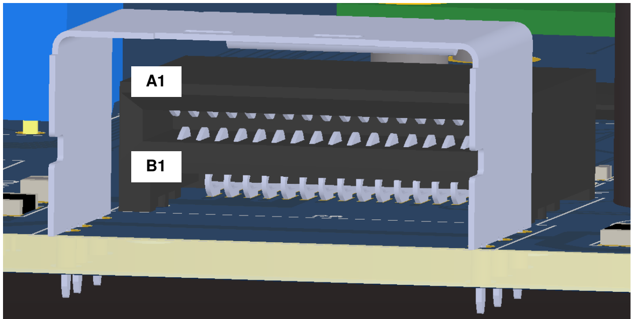
Figure 9 – P8 Remote Display I/F Connector – End View
